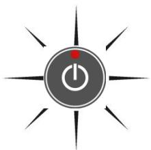
In the case of major changes to the mounting position (e.g. accidentally moving the tripod leg), a TILT function ensures that the device switches off and draws attention to the fact by the laser beam and the levelling LED flashing quickly.
