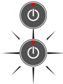
The Laserbeam and the levelling LED is blinking. If the tripod head is sloping by more than 5°, this is indicated by the laser beam flashing quickly and the Level LED.
